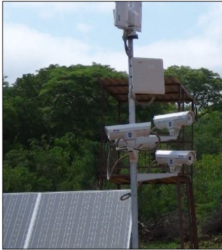
Fig. 10. Solar-powered camera array guarding the mining road that connects the Pink and Red Zones.
