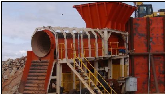
Fig. 6: Trommelscreen to concentrate the ore.
