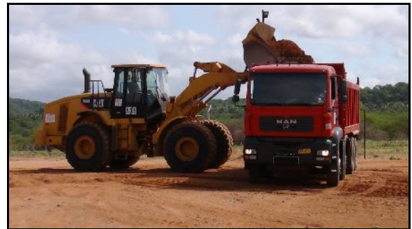
Fig. 7: CAT front loader scooping the concentrated ore on MAN dump truck.
